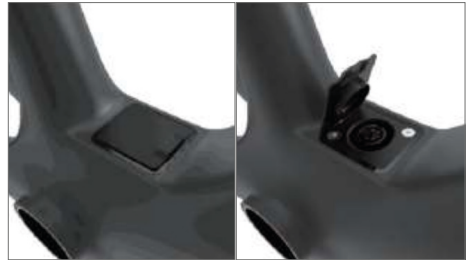
Position of charging port and dedicated lid.
